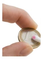
Chemo Nickel Test™ (NT) and Chemo CobaltTest™ (CoT) are one-component solutions that enable easy detection of free nickel or cobalt in metallic objects.
